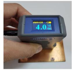
milum mm125 rechargeable battery operated handheld copper thickness gage. Can accurately measure Printed Circuit board laminate copper thickness with digital display showing Oz value. Measures complete range of copper thickness. Simple to use and easy to hold. Long life rechargeable battery is economic and environmental.
